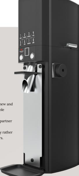
Self-service, high-volume commercial and industrial use **Target application** Disc diameter Disc lifetime\* 120 mm 15-20 tons Alternating current (AC); commercial three-phase power supply **Motor technology** 2.5 kg / 5 lbs per minute Turkish fine to cold brew **Grinding output\*** Grind size range Manual Digital automatic **Adjustment options Hopper capacity** 2.5 kg 37 kg (net) 250 x 810 x 320 mm Weight Dimensions (W  $\times$  H  $\times$  D) **Standard colors** black MSRP (CHF) 4.700
